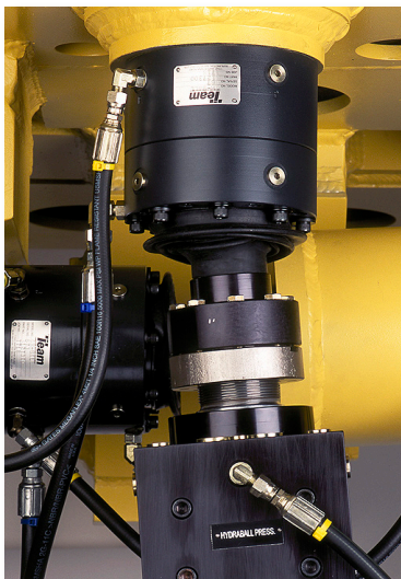
HydraBalls on both the MANTIS™ actuator and drive link.
