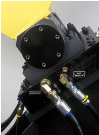
Hydrostatic rotary bearing provides pivot for lateral bell cranks.
