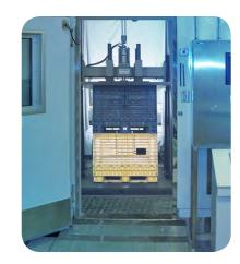
Climatized Testing Temperature and relative humidity can greatly impact compression performance of your packaging designs. To replicate these conditions during testing, Lansmont Compression Test Systems can be installed inside a climate-controlled space.
