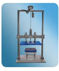
**Testing Individual Packages** For testing smaller items such as individual packages, an optional package test stand can be used with the Model 152. A Low Range Load Platform is another useful option for accurately evaluating low level force inputs.
