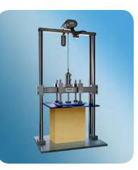
Testing a Unit Load Lansmont's Model 152 Compression Tester is specifically designed to efficiently and accurately evaluate the performance of unit loads under compressive forces.
