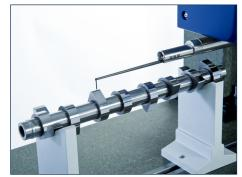
High range, high resolution systems for contour and surface finish measurement
