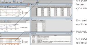
It is possible to confirm the input waveform, stress-strain curve, and various parameters for each acquisition cycle. Data for any specific point can also be extracted from any cycle waveform using the point picking function.
