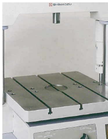
Optional Surface Plate Allows Full-Scale Testing
