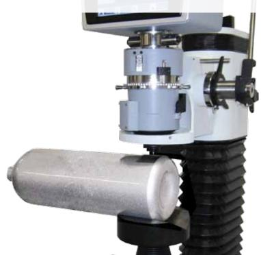
Measuring on components of large dimensions is possible. In this case the indenter has an extension of 50mm.
